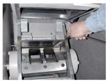
Figure: Checking the knife gap
